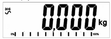
• The scale has an automatic re-zeroing function to account for minor drifting or accumulation of material on the platform. However you may need to press the [→0←/Esc] key to re-zero the indicator if small amounts of weight are shown when the platform is empty.
