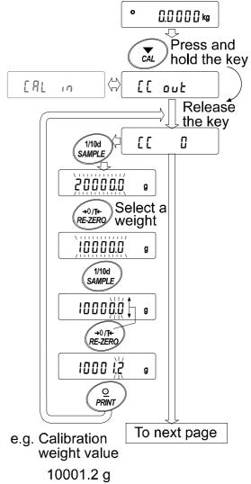
5 Confirm that there is nothing on the pan and press the PRINT key. The balance measures the zero point and displays the measured value. Do not allow vibration or drafts to affect the balance.
