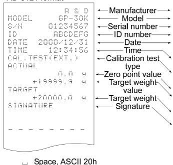
MODEL\_\_\_\_GP-30K<TERM> S/N\_\_\_\_01234567<TERM> ID\_\_\_\_ABCDEFG<TERM> DATE<TERM> \_\_\_\_2000/12/31<TERM> TIME<TERM> \_\_\_\_12:34:56<TERM> CAL. TEST (EXT.) < TERM> ACTUAL < TERM> \_\_\_\_\_O. O\_\_g<TERM> \_\_\_\_+19999.9\_\_g<TERM> TARGET<TERM> \_\_\_\_+20000.0\_\_g<TERM> SIGNATURE<TERM> <TERM> <TERM>
