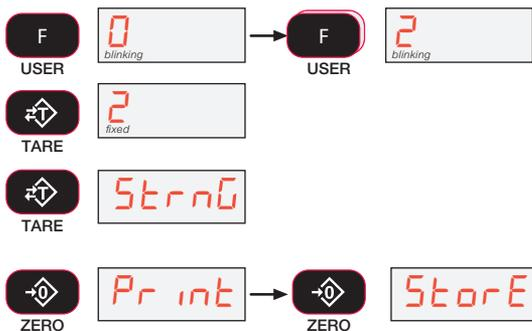
Figure 7-4. Printer Output Setup
