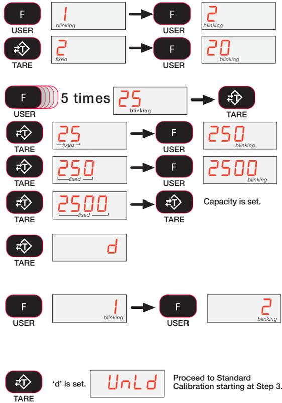
Figure 5-5. Initial Calibration
