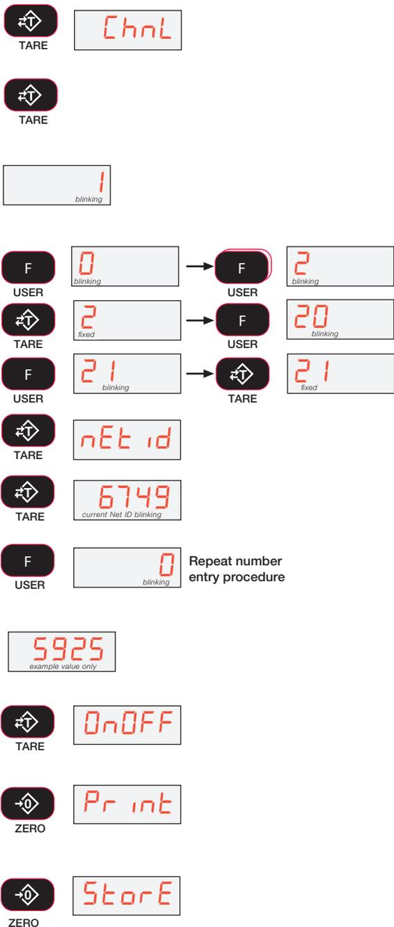
Figure 7-7. RF Setup Procedure
