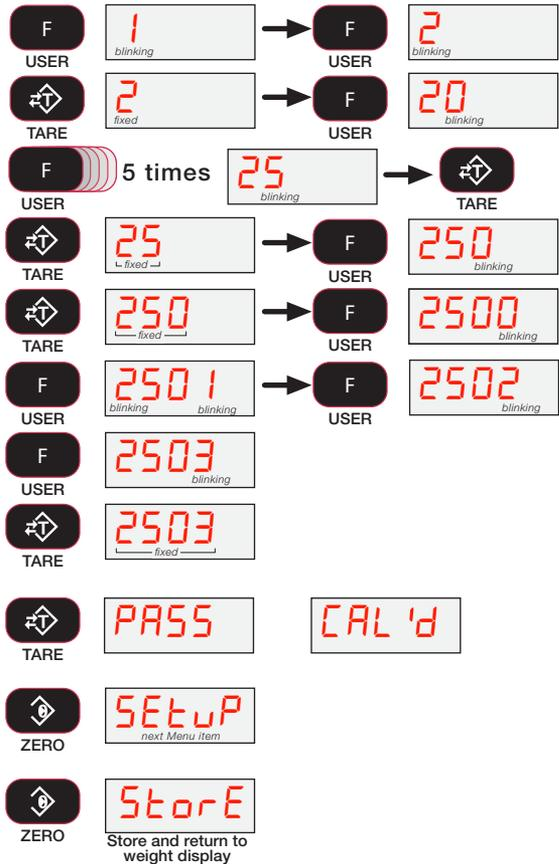
Figure 5-7. C-Cal Calibration Procedure
