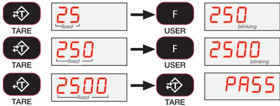
11) The display now reads **Load2**. The 3460 allows multipoint calibration. If more cal points are desired (up to 3 additional) press **TARE**. If a single point cal is all that's needed, press **ZERO** and jump to step 15.
