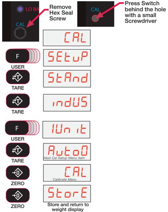
Figure 5-9. Weight Standard Setup
