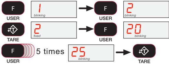
10) When the entire value of the test weight is displayed and the weight and scale are stable, press **TARE** to finish off the weight entry. If the resultant cal value is within limits, the display will read **PASS** briefly.
