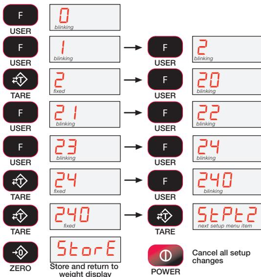
Figure 4-7. Setpoint Setup
