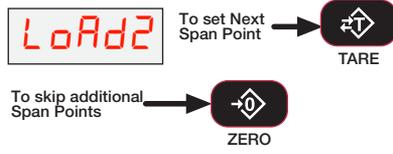
12) Load the scale with the next test weight. The display offers the reading that will occur without adjusting the value. If the weight value shown is acceptable push **TARE** and skip to step 14. If the calibrated value needs adjusting, go to step 13.
