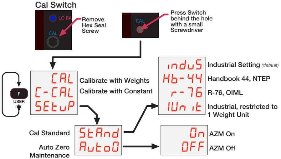
Figure 5-8. Calibration Setup
