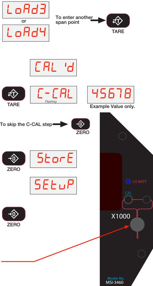
Figure 5-3. Standard Calibration Procedure
