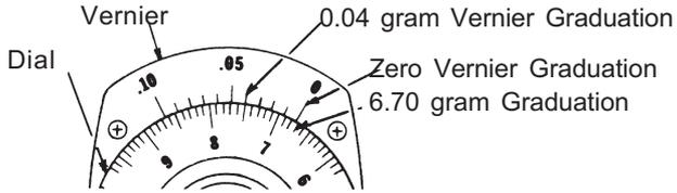
Figure 8. Vernier Dial Reading of 6.74 Grams.
