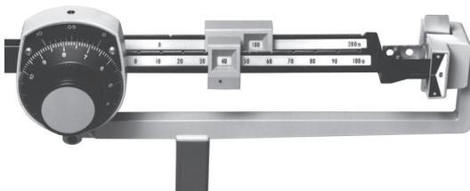
Figure 7. Example of 146.74 Gram Reading.
